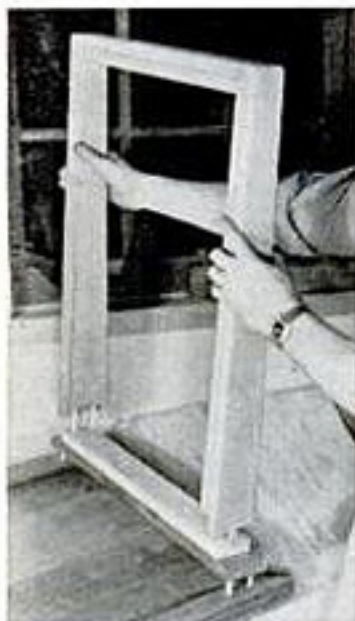
Method of fastening end leg, shown at left, insures it against wobble since it virtually becomes a single structure with the top.
